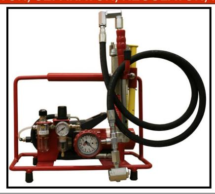
The most common issue with the **QS-2000A** is damage to the Enerpac pump due to dirty or wet air. A re-kit and repair of this problem is \$300-\$400 not including the cost of downtime, freight, and aggravation. Part number 2010 Regulator, Separator and Lubricator package will dramatically extend the life of the hydraulic pump and reduce downtime for only \$150.00.
