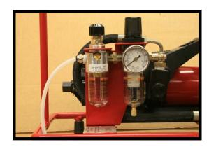
Part number 2010 Regulator, Separator and Lubricator package comes complete with bracket, hardware, air fittings, and tubing. We will install it on a new unit at no charge if both are ordered at the same time. It can also be installed easily by the operator with the use of simple hand tools.
